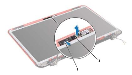
1 camera module cable connector 2 camera module
