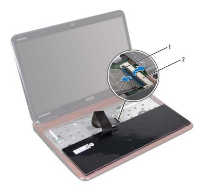
1 keyboard cable 2 keyboard-cable connector
